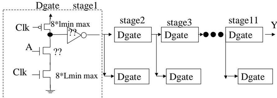
For the 11 stage circuit above, size via simulation the output inverter, and the NMOS pulldown of the DGATE such that the A to Y average delay is within 10% of the minimum delay with the lowest dynamic power consumption. You must not exceed the maximum sizes shown on the precharge/eval transistors. Your clock can be any duty cycle you wish. Note that all DGates are the same size. Use 100 ps rise/fall times on both A, Clk signals. Use Leda 0.25u, Vdd = 2.5. (note: Lmin = .25u).
