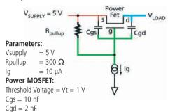
For a given power supply voltage, Ig and Cgd define how soon it can ramp up to its full scale, based on the following: **dV/dt = Ig/Cgd**
