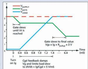
The selection of the MOSFET must be done with care and knowledge of system requirements. Care must be taken also when selecting Rpullup. If the Rpullup is too large, then the Vgs rating of the MOSFET could be exceeded, leading to catastrophic failure.
