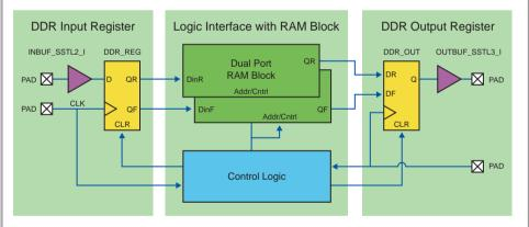
The data enters the FPGA through a pad and is captured into a DDR register, which splits the data into two outputs: QR and QF. QR is the output at the rising edge of the clock and QF is at the falling edge of the clock. The data is registered into a dual-port SRAM in Actel's ProASIC®3 FPGA. Control logic circuitry is used to control the address space to write data coming from DDR I/O registers to SRAM blocks inside the FPGA for internal processing.
