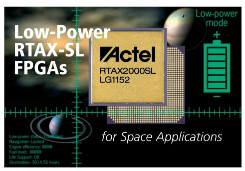
Extending its low-power offerings to the space community, Actel has developed the radiation-tolerant RTAX-SL low-power grade option field programmable gate array (FPGA) specifically targeted at high-reliability space-flight designs.
