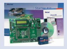
The Evaluation Board hosts the AFS600-FG256 device, with selectable voltage sources, LCD display, prototyping headers, and a 40-pin daughter card connection. It comes with FlashPro3, an in-system programmer, Libero IDE Gold "which supports all Actel devices up to 1 M system gates" and a User's Guide, tutorial schematics, and design files.
