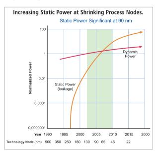
to choose technology that allows better power choices at each level of design. Choosing the lowest power FPGA or choosing a device with built-in smarts to allow your system to manage power, becomes another level of learning for the ever evolving design engineer.
