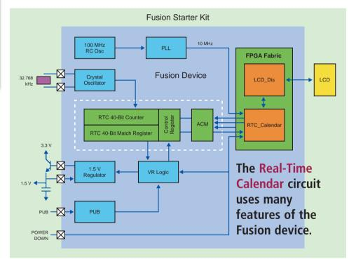
Using a 32.768 Hz crystal oscillator, with built-in prescaler, provides a 256 Hz input to the Real-Time Counter, which gives the 8th bit a 1 Hz frequency. The 40-bit counter can count for over 136 years.
