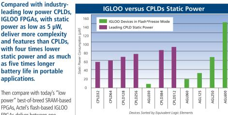
hundred and one thousand times improvement in power reduction. This two to three orders of magnitude lower static power consumption can translate into weeks and months of standby battery life. Use the Power Calculator or SmartPower links to see how IGLOO will perform in your design.
