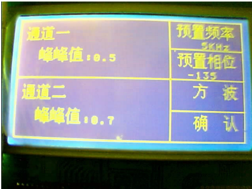
Figure 30. Self-Measured Signal Frequency Phase Setting
