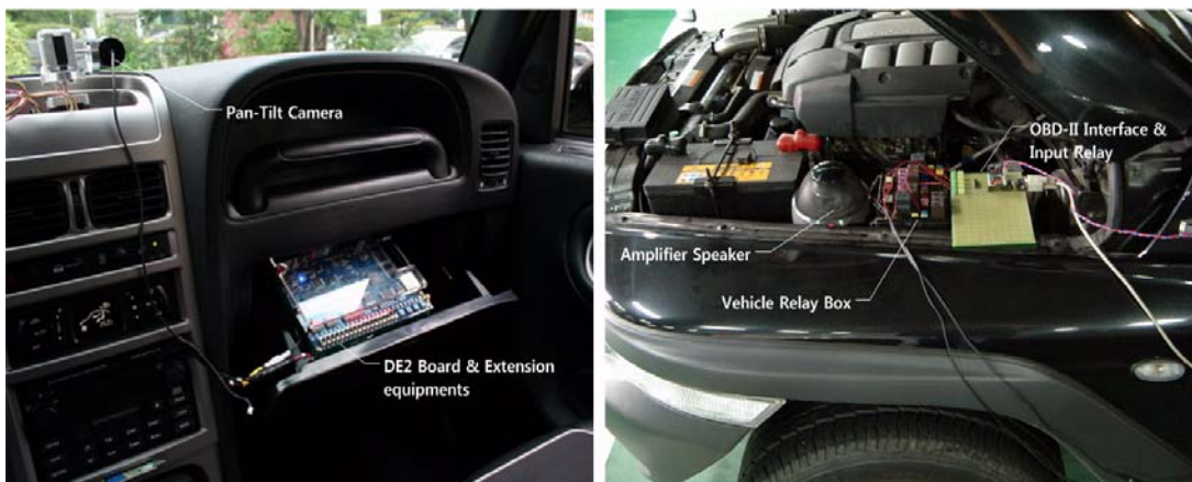
Figure 4. In-Vehicle Embedded System Configuration
