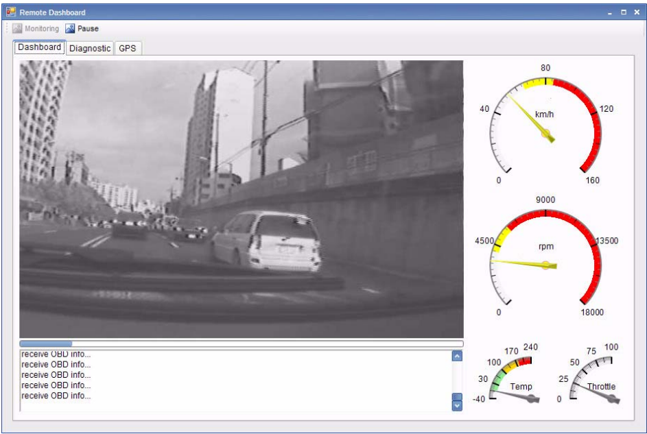
Figure 9. Captured Image and OBD-II Information Display
