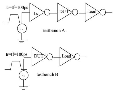
Assuming that the DUT is varied between 1X and 6X, and LOAD is varied between no-load and 6X, what would you expect the NOLOAD delay measurements for DUTs 1X to 6X to do?
