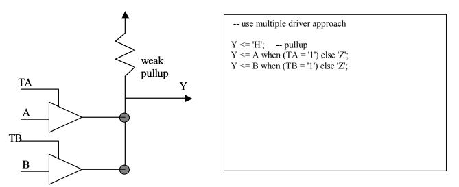
When tristate control is '1', then output follows input else high impedance output.
