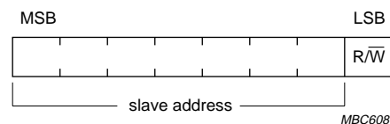
Fig.14 The first byte after the START procedure.
